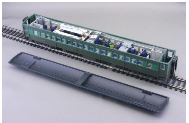
Figure 2 shows the same car with the roof removed displaying the interior and lighting. The latter operates with a reed switch and uses a AAA battery which has been removed for storage. Looking closely, one can see that the roof attaches to the carbody with a single 2-56 screw and 5/16' Plastruct channels that are cemented in the middle of both the roof and the carbody.
