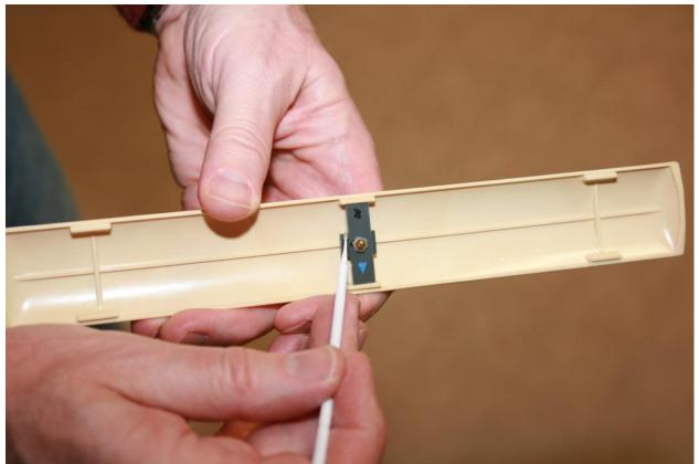
Figure 6 shows the small piece of channel being positioned on the roof channel using a 2-56 screw; a nylon hex nut was used as a spacer so that the screw didn't hit the underside of the roof. The two pieces of channel were then cemented with good old Testors. After the cement had set, the screw was removed.
